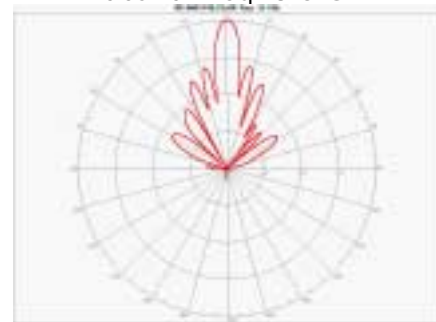
Elevation Radiation Pattern Midband Freq. 3.5 GHz
