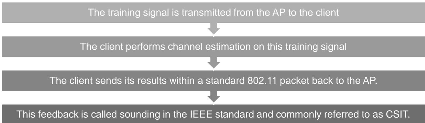
The 802.11ac beamforming improves the performance of the underlying protocol by 2 to 6 dB. However, before rushing to deploy the 802.11ac beamforming, there are several things one may want to know about it.
