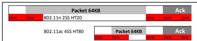
To make matters worse, there is no provision in the 802.11ac standard (unlike the 802.11n) for a Greenfield deployment. So, even in a theoretical deployment, where all the clients support 802.11ac, the non-data speeds will remain the same.
