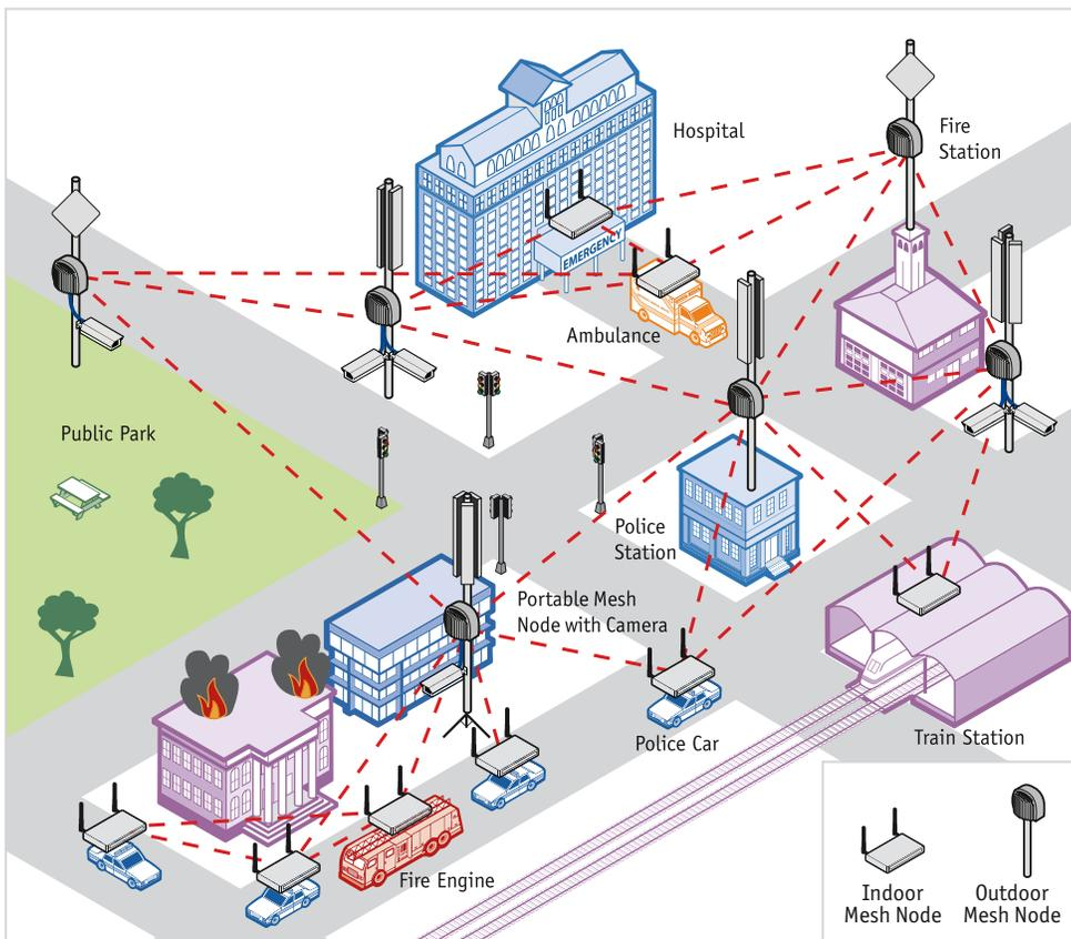
*The Firetide HotPort mesh networks provide a reliable, high-performance wireless infrastructure for public safety jurisdictions. Instant deployment and mobility also enables first responders to set up temporary incident response communications at the scene of an incident.*
